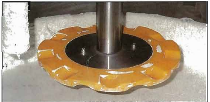
Blade mounted with stiffening plates shown after 15 months in a 40% TiO 2 slurry.
