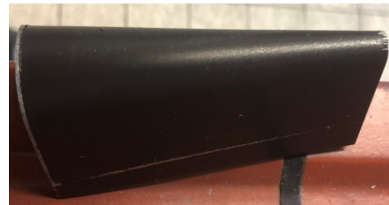
Bending elasticity of coating film baked at 450C
