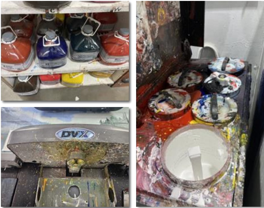
Figure 16. Traditional colorant tint system colorants (top left), dispenser (bottom left), and canisters (right)
