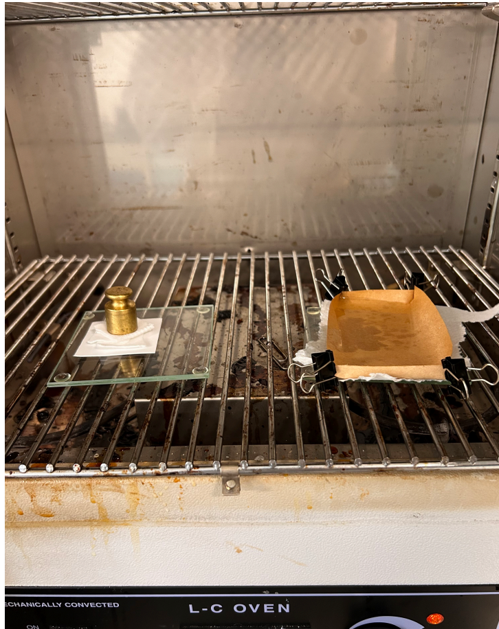
Two samples in the Oven Left sample: ASTM F119-8 Right sample: Oil-boat test
