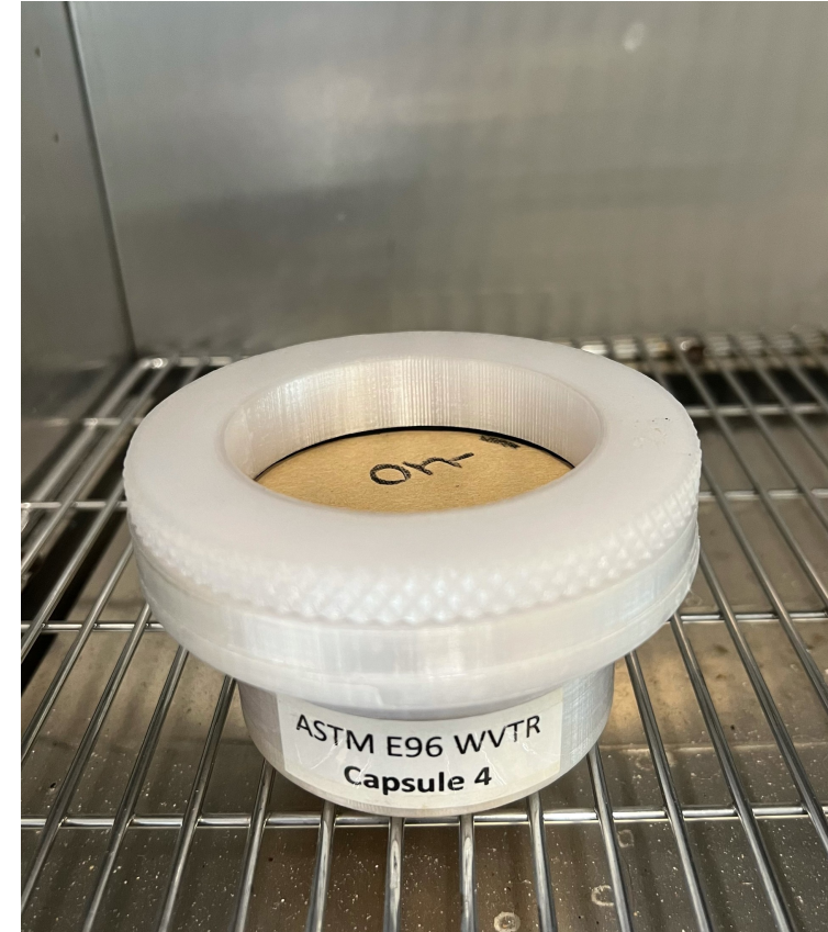
ASTM E96 MVTR: used to measure water vapor transmission rate
