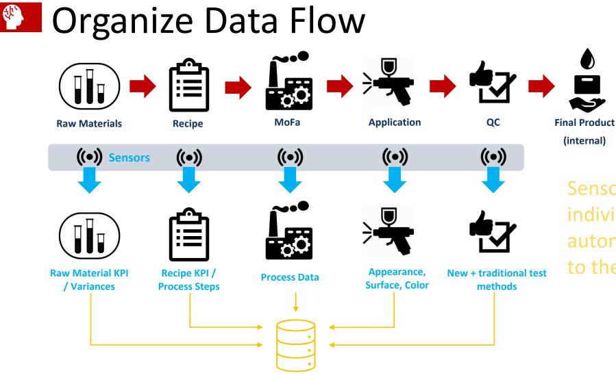
Sensor data from the individual process steps is automatically transferred to the cloud database.
