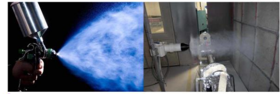
FIGURE 1. Gun 1 vs. bell 2 atomizers
