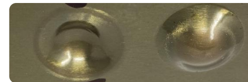
Impact (160lbf) front and backside
