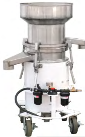
Pneumatic Model RBF-15 with feed hopper weldment
