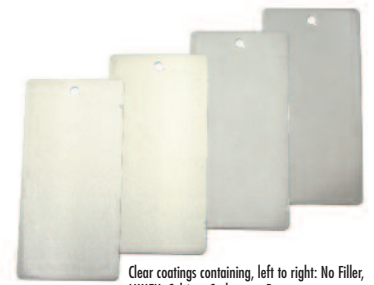
Clear coatings containing, left to right: No Filler, MINEX, Calcium Carbonate, Baryte.
