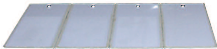
Powder coatings subjected to QUV exposure and containing, left to right: Calcium Carbonate, Baryte, Wollastonite, MINEX.
